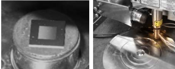
▲ Standard test sample grid on Veeco Multimode™; ▲ Search over millimeters via mechanical positioners or motorized platter
